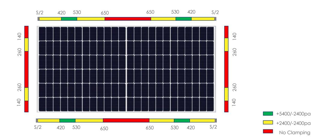
RSM40-8-xxxM/N Clamping Zone Diagram
